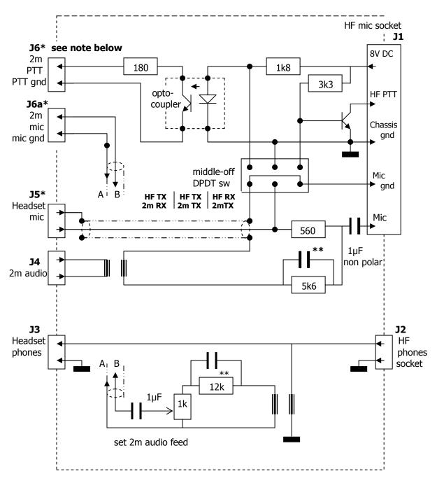
J1: 8-pin mic socket Dotted line: Aluminium diecast box
